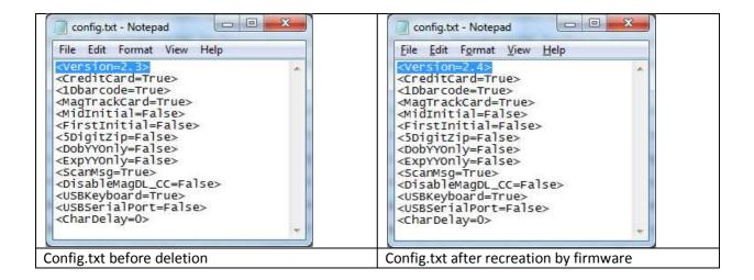
Tip – Backup all the files on the TokenWorks drive before doing any updates. In the event the new firmware doesn't run as expected, delete all the files and use the backups to manual update the new files as the OS may be looking for new parameters in new versions of the file.
