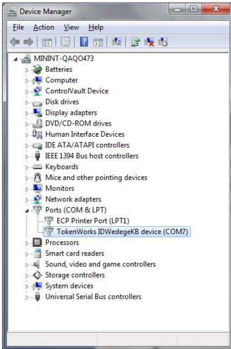
The PC has selected COM7 for this PC. The Chrome Extension Serial Port test app uses ports 1-9, so if your installation selected a higher port, you can change this by right clicking the entry in the device manager and select properties, then select Advanced on the properties page, and select a lower com port:
