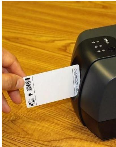
*Calibration card inserted with arrow facing outward*
