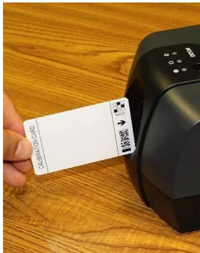
*Calibration card inserted with arrow **facing inward***
