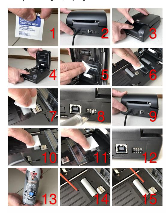
Leave the unit open for a minute for the moisture to dry, close the lid, and then power it on. The 150 ID scanner is now ready to use.
